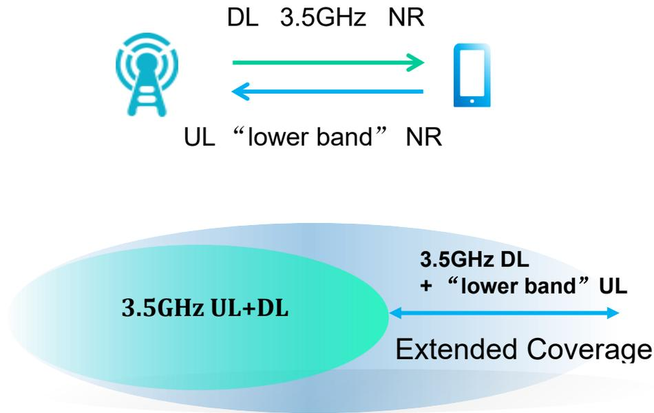
**Figure 4:** An example solution of extending 5G-NR coverage by combining C-band and a lower band.
